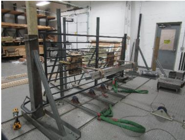
Photo No. 3 In-Fill Load Test at Center of Two Horizontal Pickets
