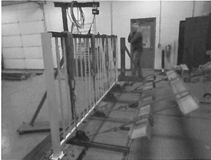
Photo No. 6 Vertical Uniform Load on Top Rail
