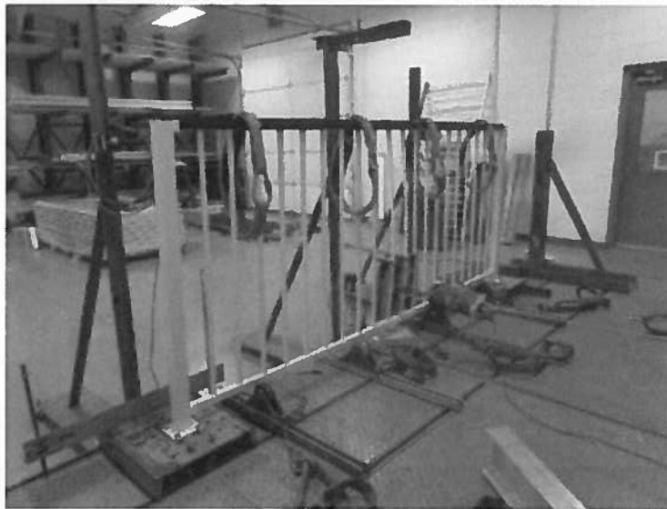
Photo No. 2 In-Fill Load Test at Bottom of Three Pickets
