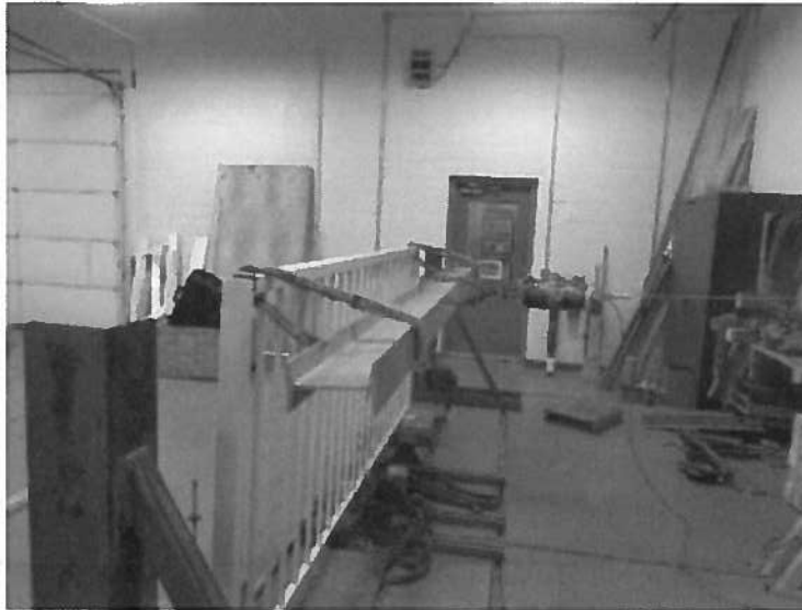
Photo No. 4 Concentrated Load Test at Ends of Top Rail (Brackets)
