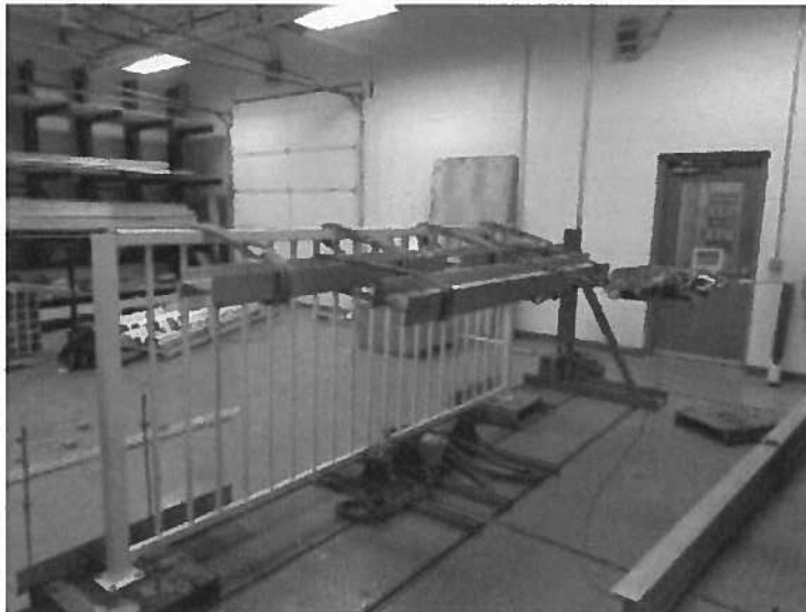
Photo No. 5 Horizontal Uniform Load on Top Rail
