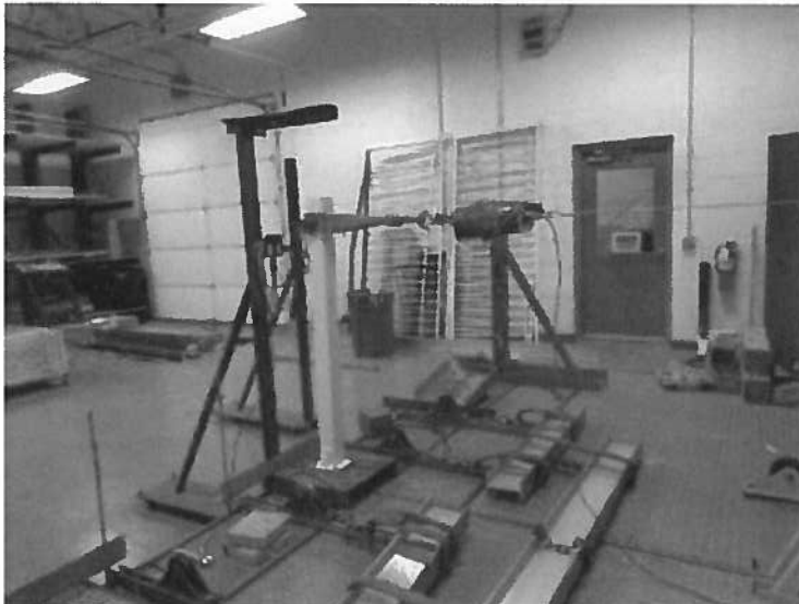
Photo No. 7 Concentrated Load Test at Top of Stand-Alone Post (42 in high)
