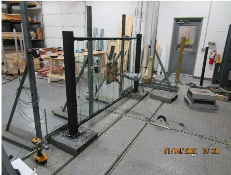
Photo No. 1 In-Fill Load Test at Center of Two Glass Balustrades
