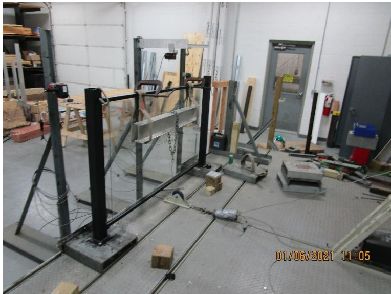
Photo No. 5 Vertical Uniform Test on Top Rail
