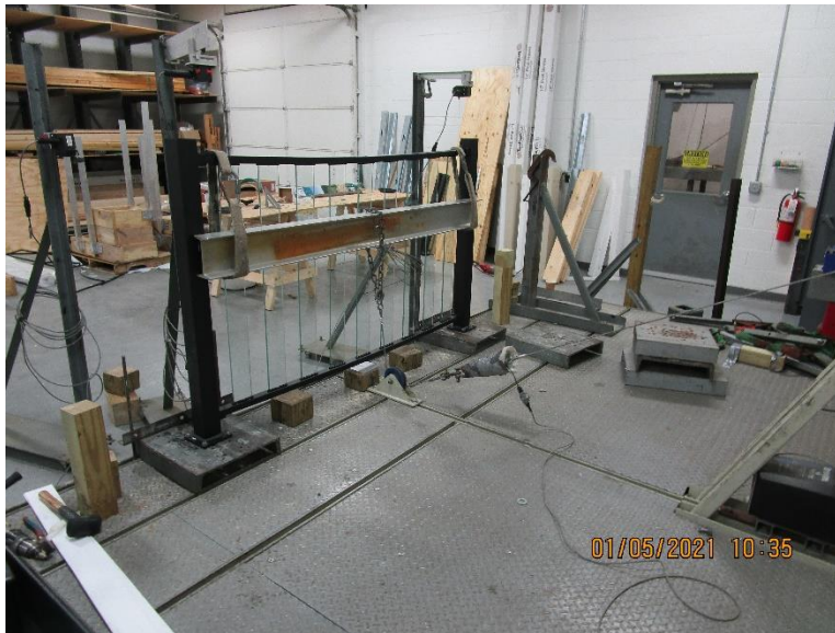
Photo No. 9 Vertical Concentrated Load at Ends of Rail (Brackets)
