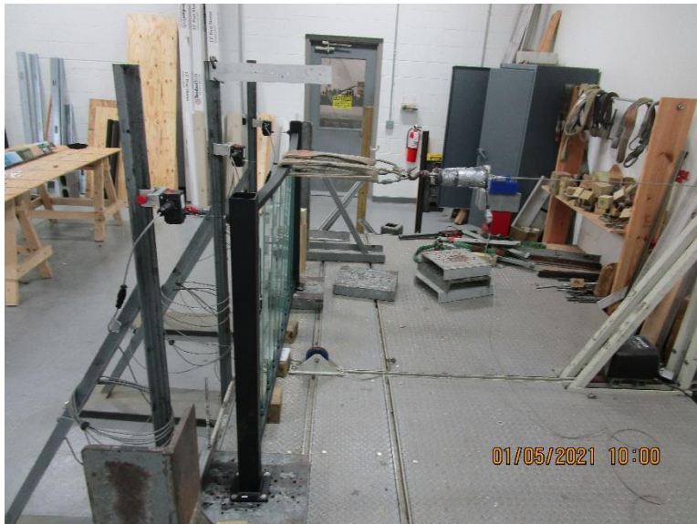
Photo No. 6 Horizontal Concentrated Load Test at Midspan of Top Rail
