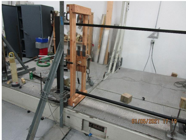
Photo No. 3 In-Fill Load Test at Edge of Glass Panel
