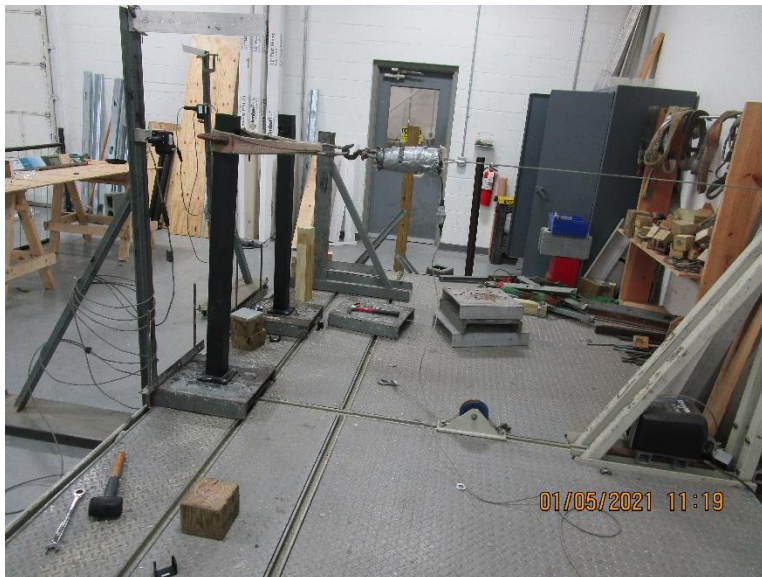
Photo No. 10 Concentrated Load at Top of Stand-Alone Post
