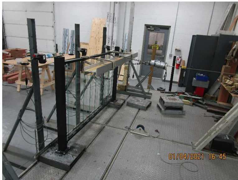
Photo No. 4 Horizontal Uniform Test on Top Rail
